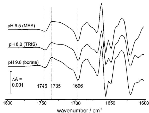
FIGURE 6: Redox FTIR absorbance difference spectra of purified cytochrome  $bo_3$  (tagged at subunit IV) equilibrated to different buffers at various pH values: 20 mM *N*-morpholinoethanesulfonic acid (MES), pH 6.5 (top); 20 mM Tris-HCl, pH 8.0 (middle); and 20 mM sodium borate, pH 9.8 (bottom).
